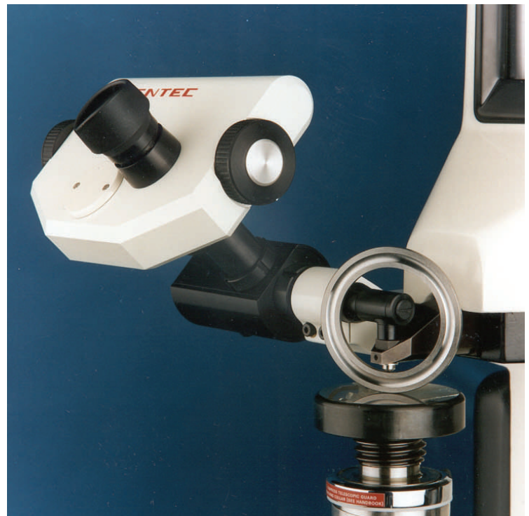
Measuring the Hardness of an Internal Bore
