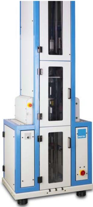
A highly versatile range of drop weight impact testers for performing a wide range of medium energy tests on materials, specimens and end products of various geometry.
