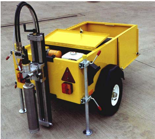
Merlin Diamond Coring Trailer, smallest In the range, cores up to 150 mm in Re-instatements and roads.
