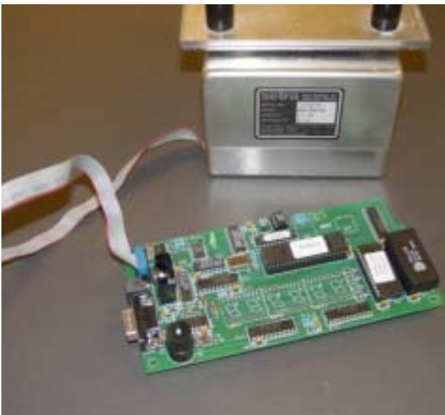
SETRA balance and display board
