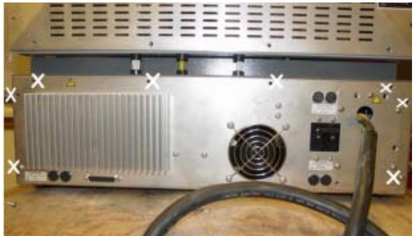
8 screws to remove to slide out control panel.
