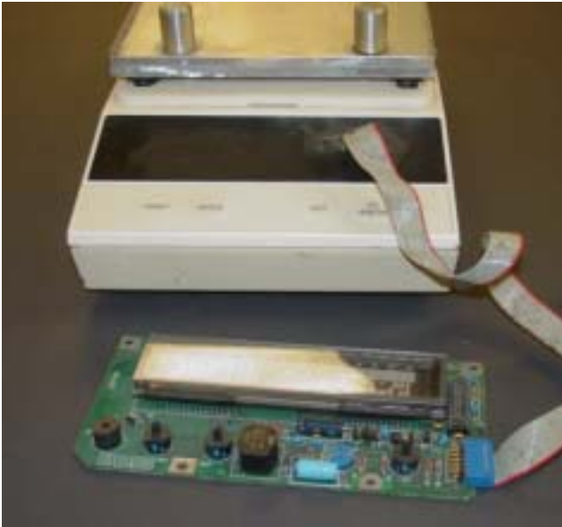
OHAUS balance and display board
