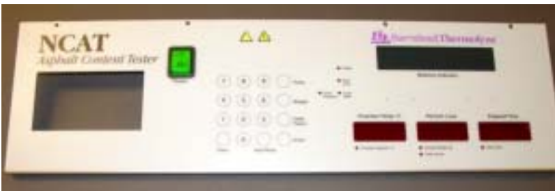
DL1275X4 keypad - 1275 series only (Martel printer)
