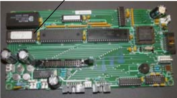
Main Logic Board - Software I.C.
